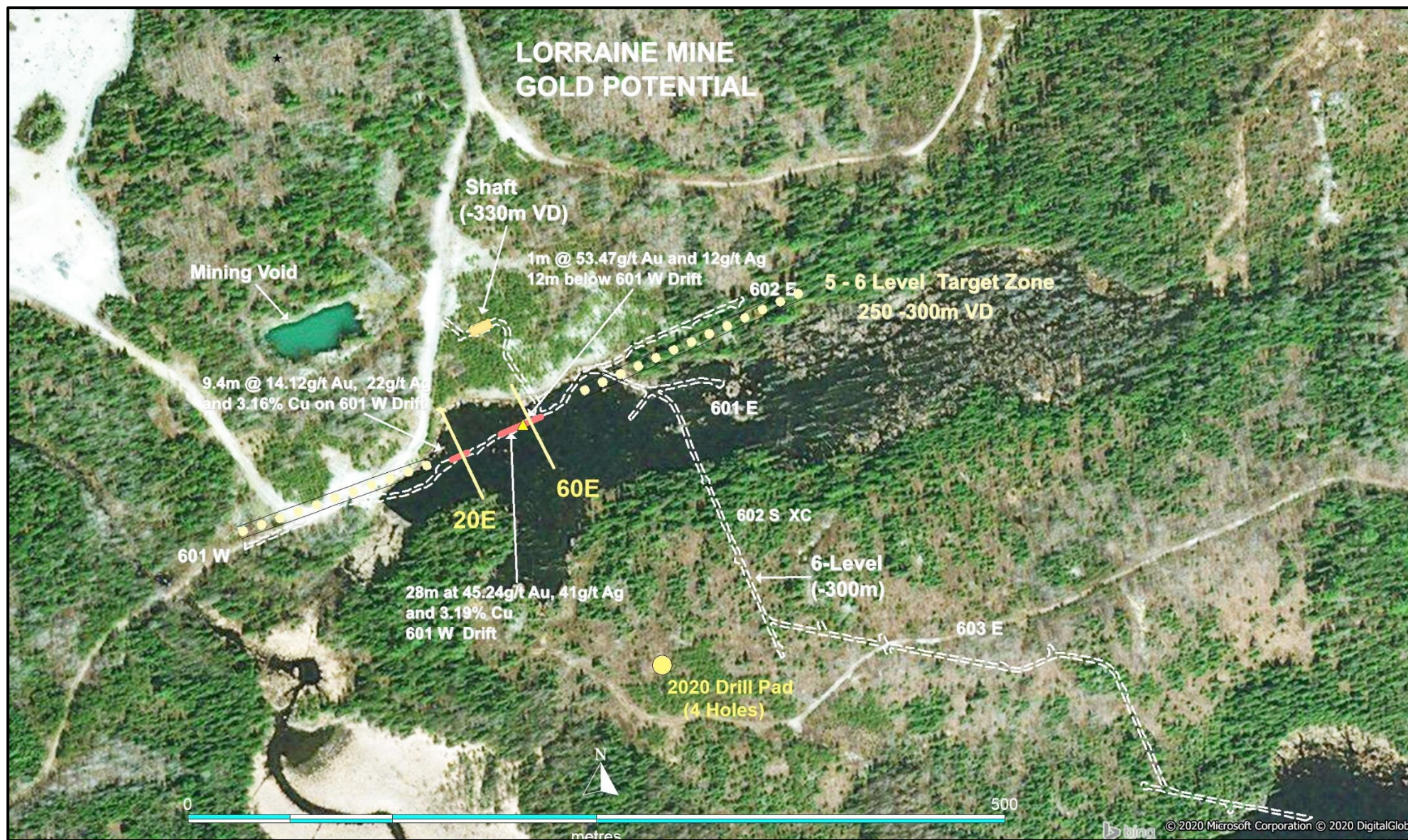
Figure 6: Lorraine Mine Site – Surface Plan with 6-Level Gold Sampling. Target Mine Sections 20E and 60E also shown.
