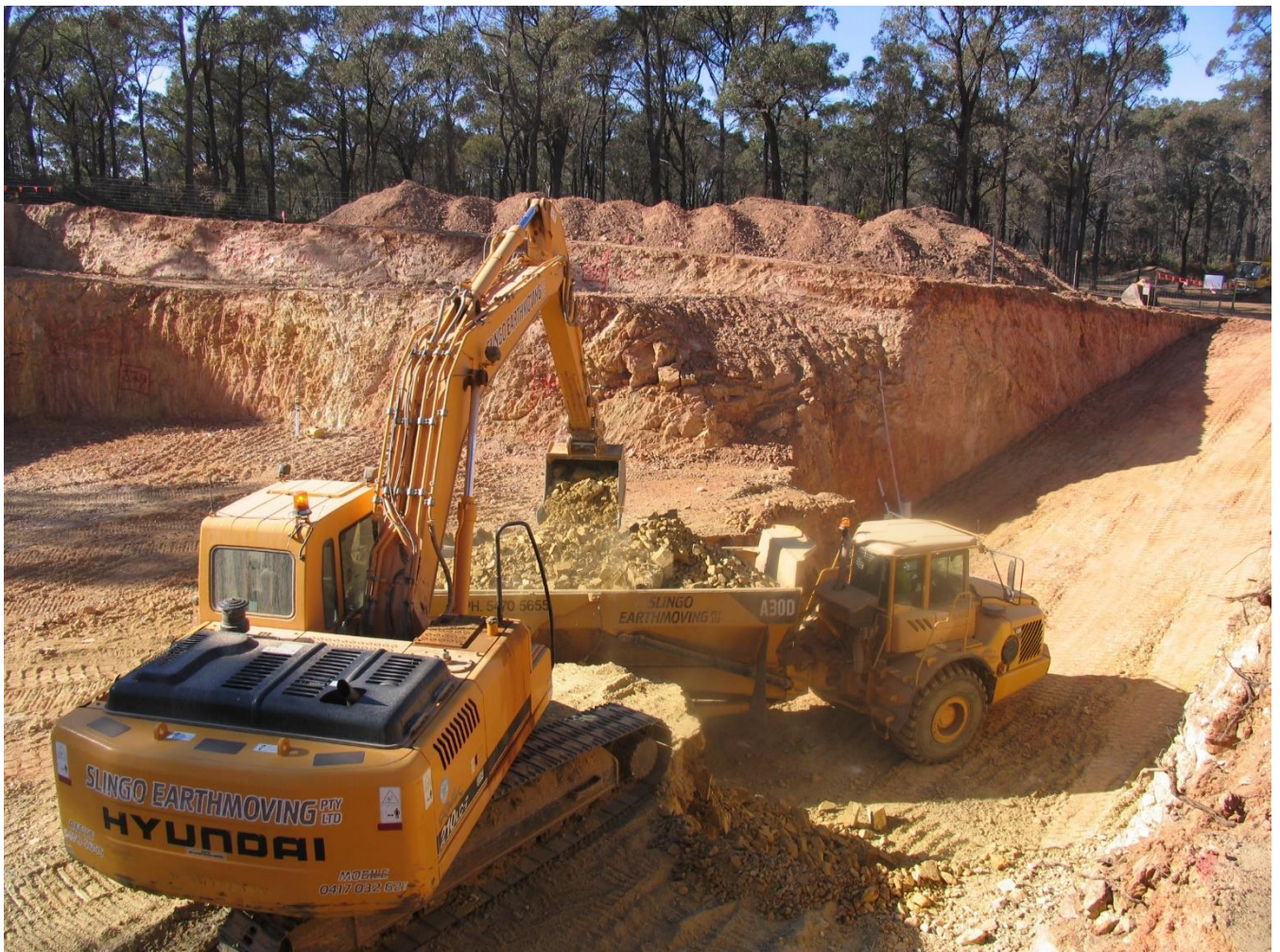
Figure 4: Excavating Bulk Sample Pit at Harvest Home
