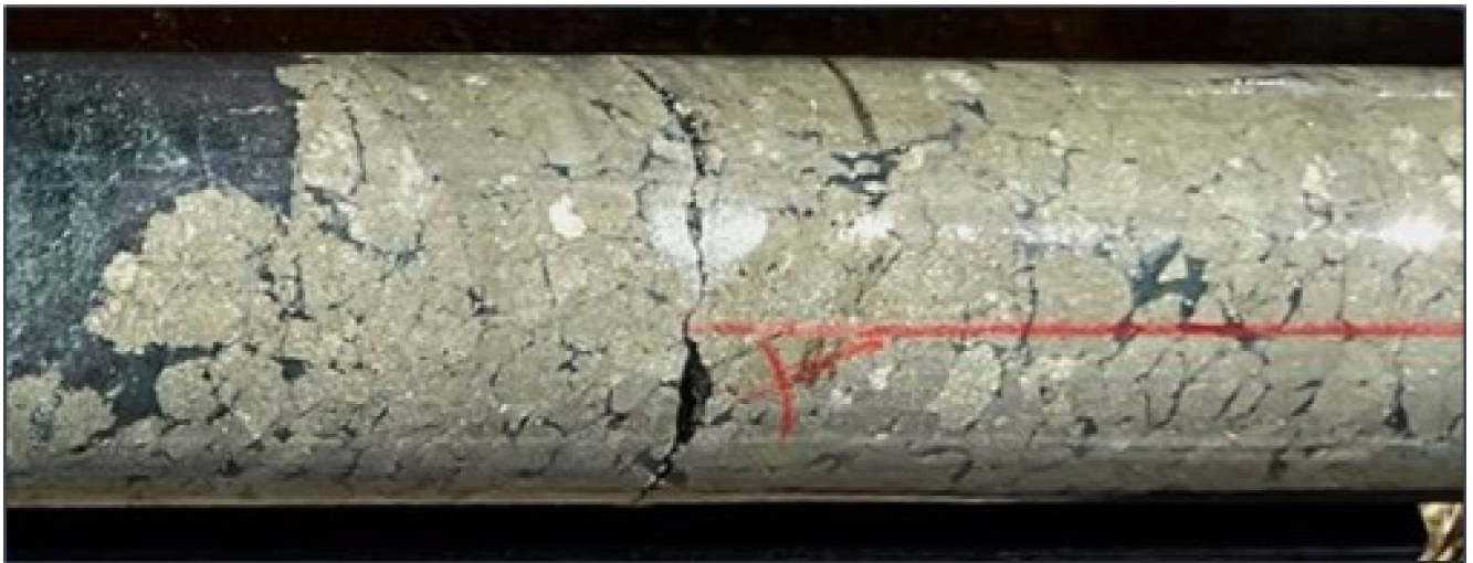
Figure 5. RMD001 massive pyrite, at 316m down hole.
