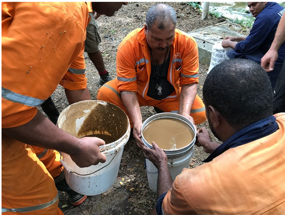
Figure 2: Lion One's Fijian crew training in method of BLEG sample treatment.
