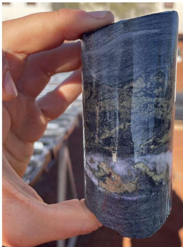
Figure 3. Copper Hills Prospect - mafic schist with chalcopyrite in quartz stringer
