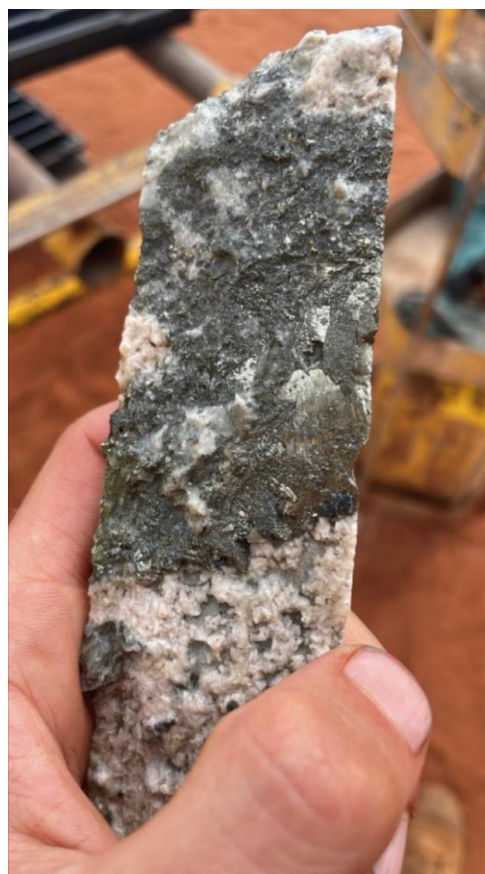
Figure 5. Goodenia Prospect – sphalerite (black mineral), in the form of marmatite a high-iron sphalerite, infilling a 5cm thick carbonate vein
