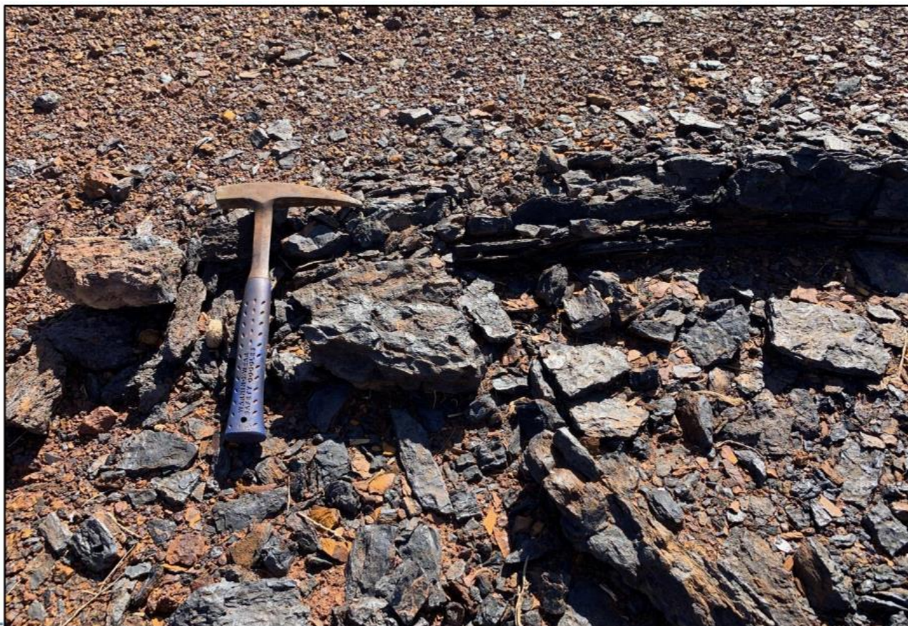
Figure 4: Manganese replacement of laminated shale at Manganese Area 3 - WR0018Mn - 36.1 % Mn from laboratory analysis (previously 26.2% Mn from pXRF)
