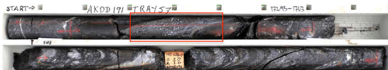
Figure 4 - AKDD191 core samples including massive galena and sphalerite within the intersection 0.7 m @ 8.5% Zn, 4.4% Pb, 32g/t Ag and 0.6% Au from 173.1 m
