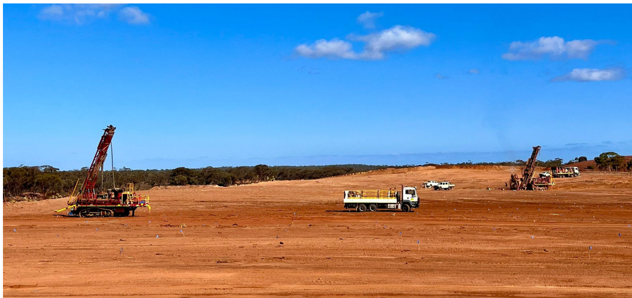
Figure 1: Grade control drilling at Fingals.
