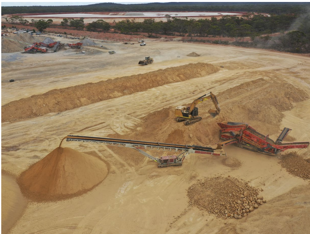
Figure 3: Screen/Stacker A-Cap oxide ore 28 January 2025
