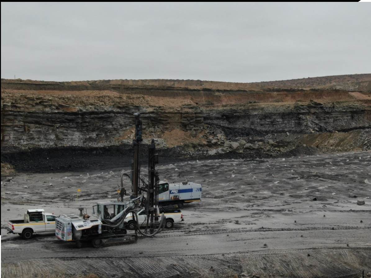
Blast Hole drilling at the Kliprand Colliery
