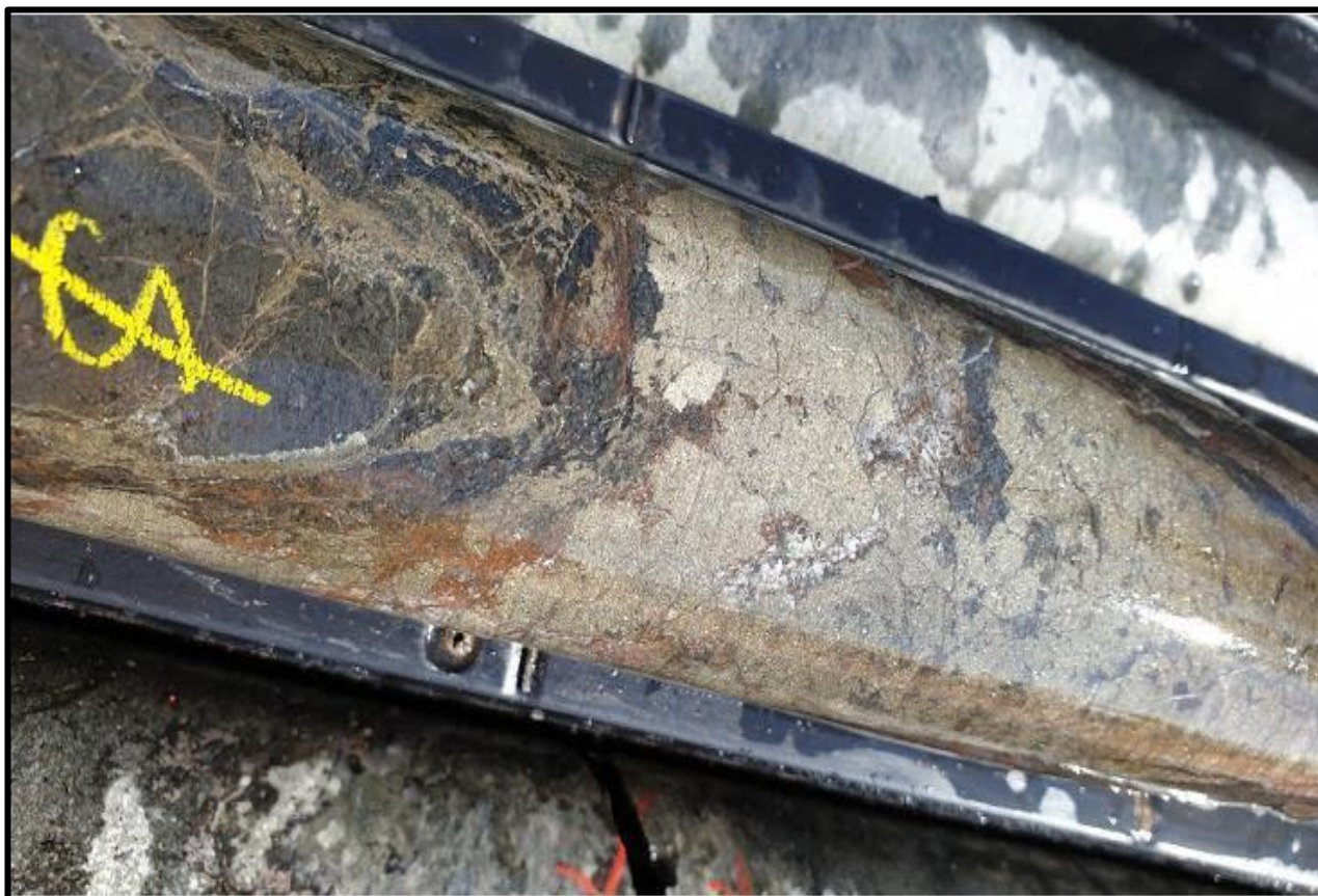
Figure 6: Semi-massive to massive pyrrhotite-pyrite vein at 331m down-hole depth in drill-hole 19AFDD1008 completed on the Hook 1 prospect.
