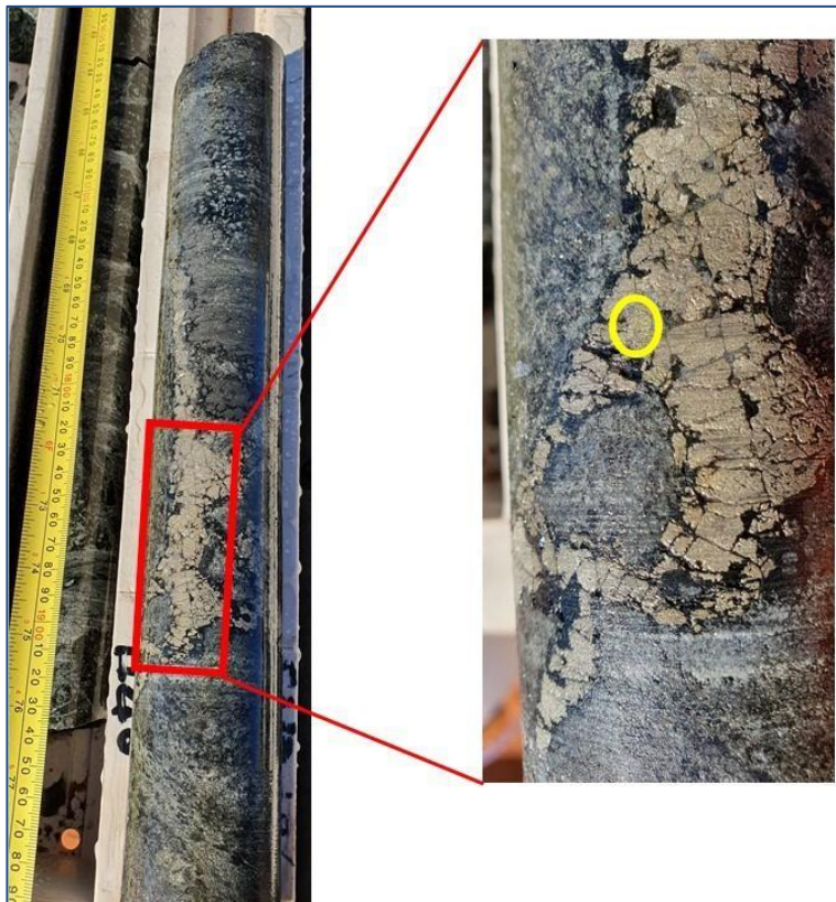
Figure 3: Semi massive pyrite-pyrrhotite vein from 188.3m-188.8m. The yellow circle indicates a chalcopyrite grain.
