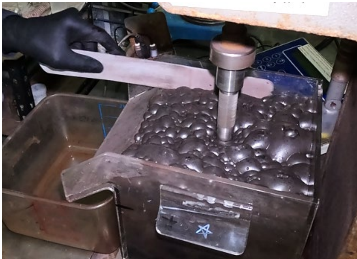
Figure 2 - Bench scale flotation testwork at Bureau Veritas laboratories, Adelaide
