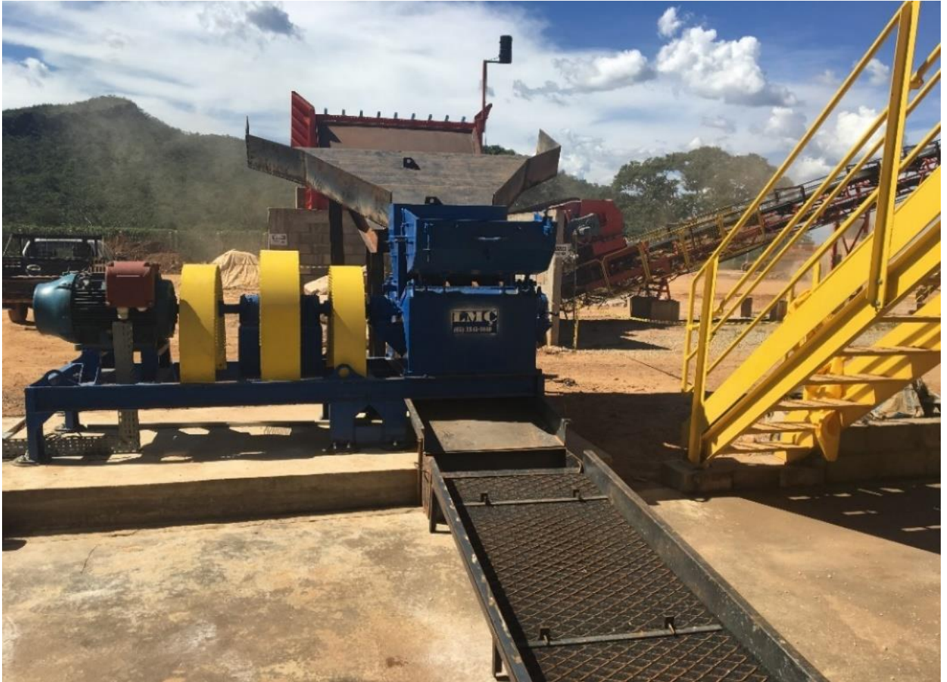
Image 3; Hammer mill installed
