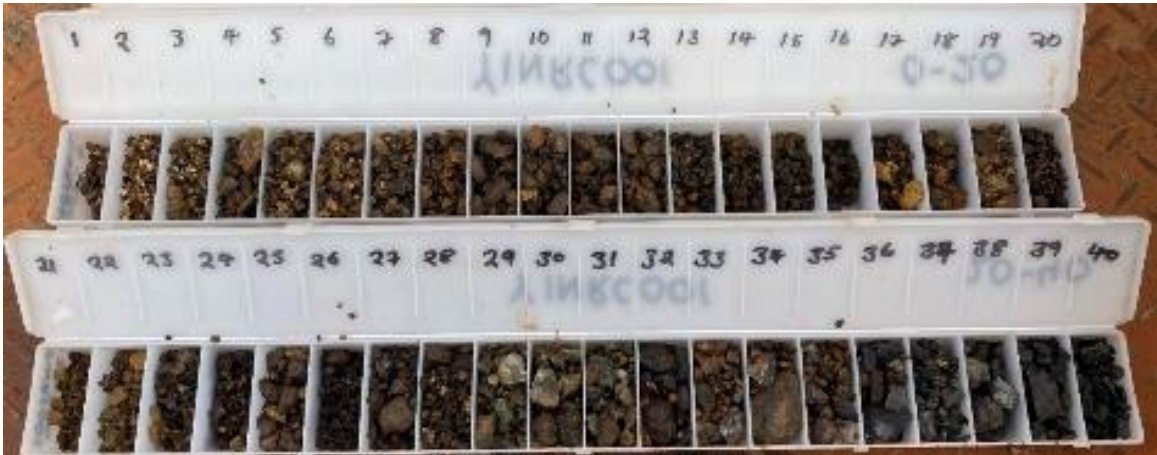
Figure 3: Chip tray from YINRC001 showing mineralised oxidized ironstone from 1-34m and grading into dark fenitic alteration.
