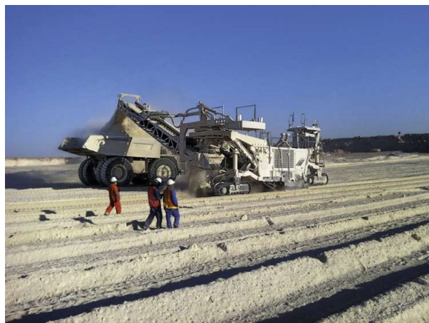
Fig 2 – Example Surface Miner – Limestone row cutting
