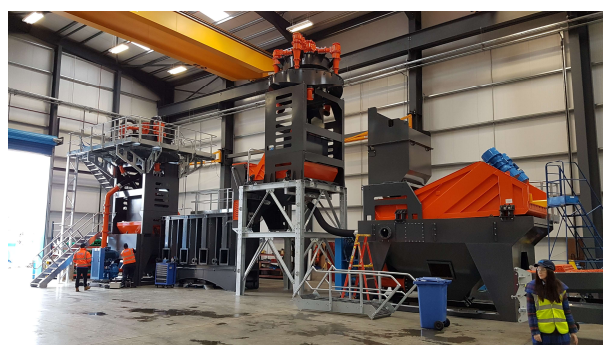
CAPTION: Trial assembly of the 70tph modular wet plant
