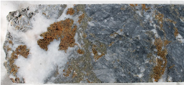
Photo 1: Millennium prospect – EPT2198 (~235.6m) Sphalerite (brown) and pyrite in brecciated carbonate. Assaying of this interval returned a grade of 6.7% zinc. Core sample width approx. 50mm
