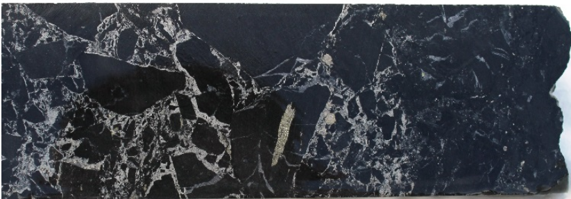
Photo 2: Millennium prospect – EPT2198 (~295m) Sphalerite (light brown) and minor pyrite in brecciated shale. Assaying of this interval returned a grade of 6.6% zinc. Core sample width approx. 50mm
