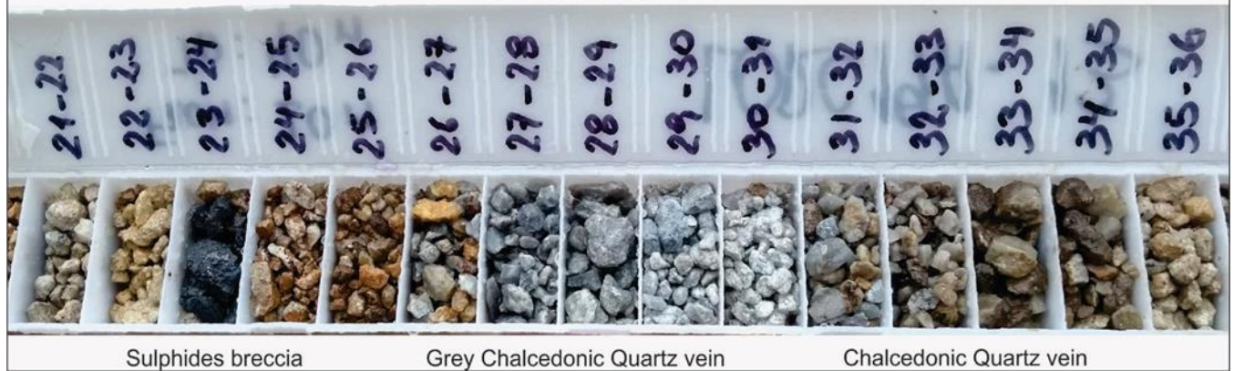
Figure 4 RC drilling rock chip samples from hole LORC19-13 from depth of 21 m through to 36m showing crystalline and chalcedonic quartz, with some banded chalcedonic quartz: pyrite sphalerite, black silica. Sulphides are interpreted to be pyrite, arsenopyrite, sphalerite, hematite and minor chalcocopyrite.
