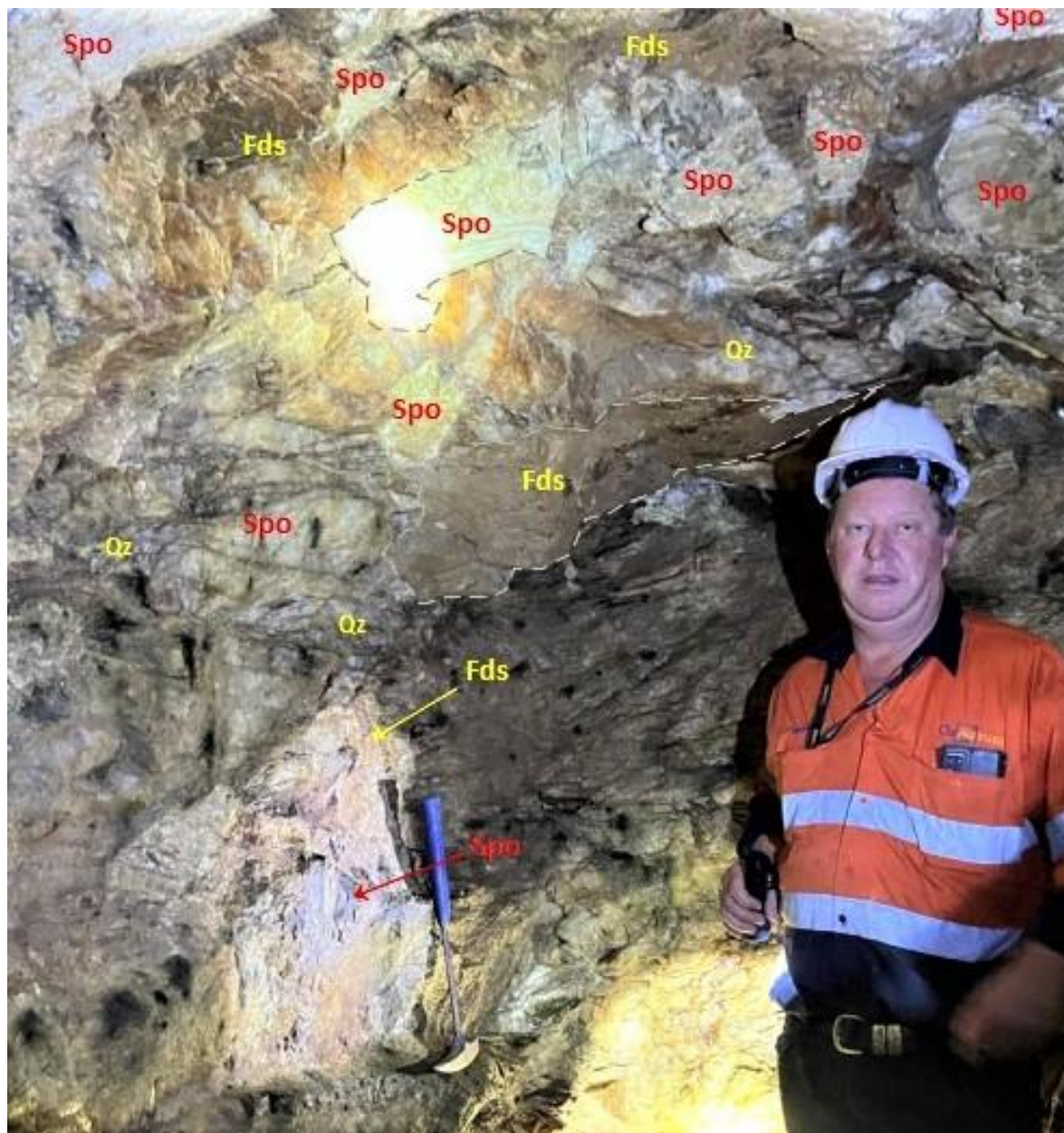
Figure 5: Coarse spodumene crystals (Spo) within Spodumene Zone in Jaime Linopolis Sítio do Estevinho underground mine. Other minerals are Feldspar (Fds) and Quartz (Qz) and black Tourmaline. Spodumene occupies at least 25 % of the field of view in this picture.
