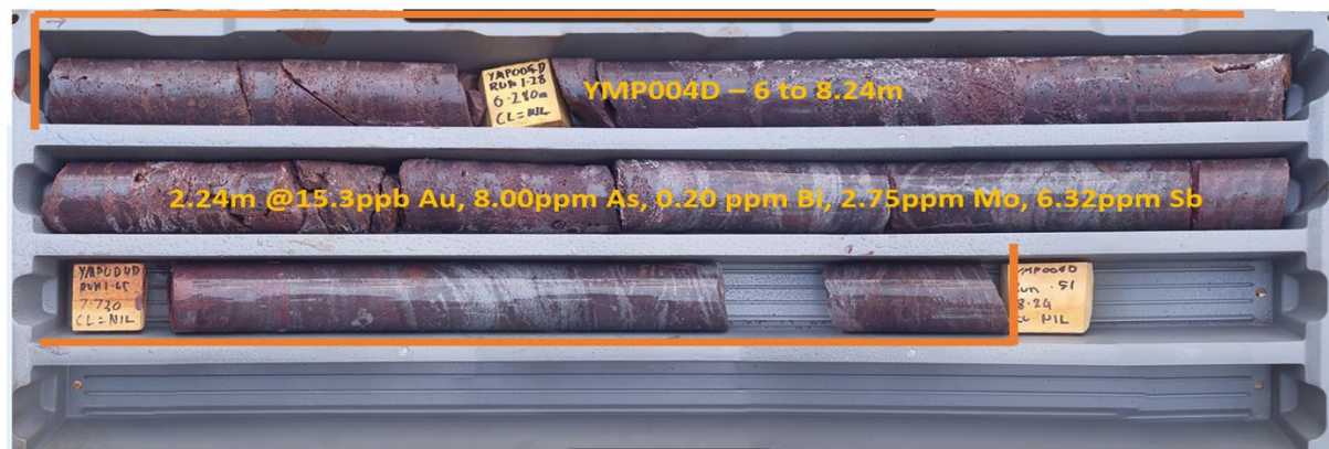
Figure 2 - Anomalous trace element geochemistry associated with hematite alteration in YMP004D.
