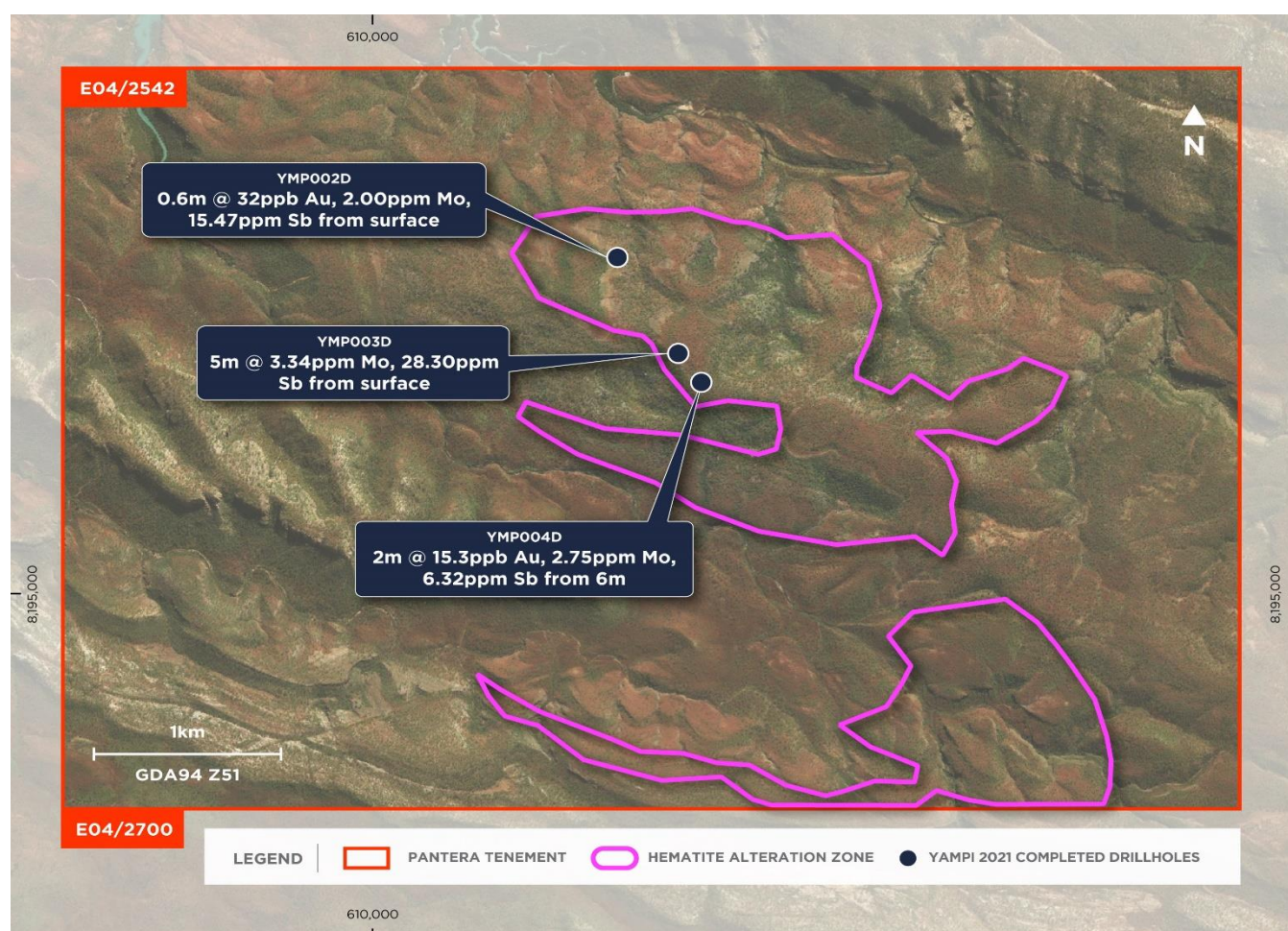
Figure 3 - Drillhole location map with anomalous trace element geochemistry. Collar details are shown in Table 2.
