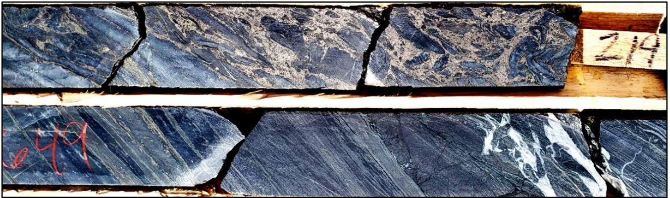
Figure 5: Hole CM-19-05 ~219m – Banded Chert / Breccia with late-stage pyrrhotite matrix and banded chert with laminated pyrrhotite replacing magnetite
