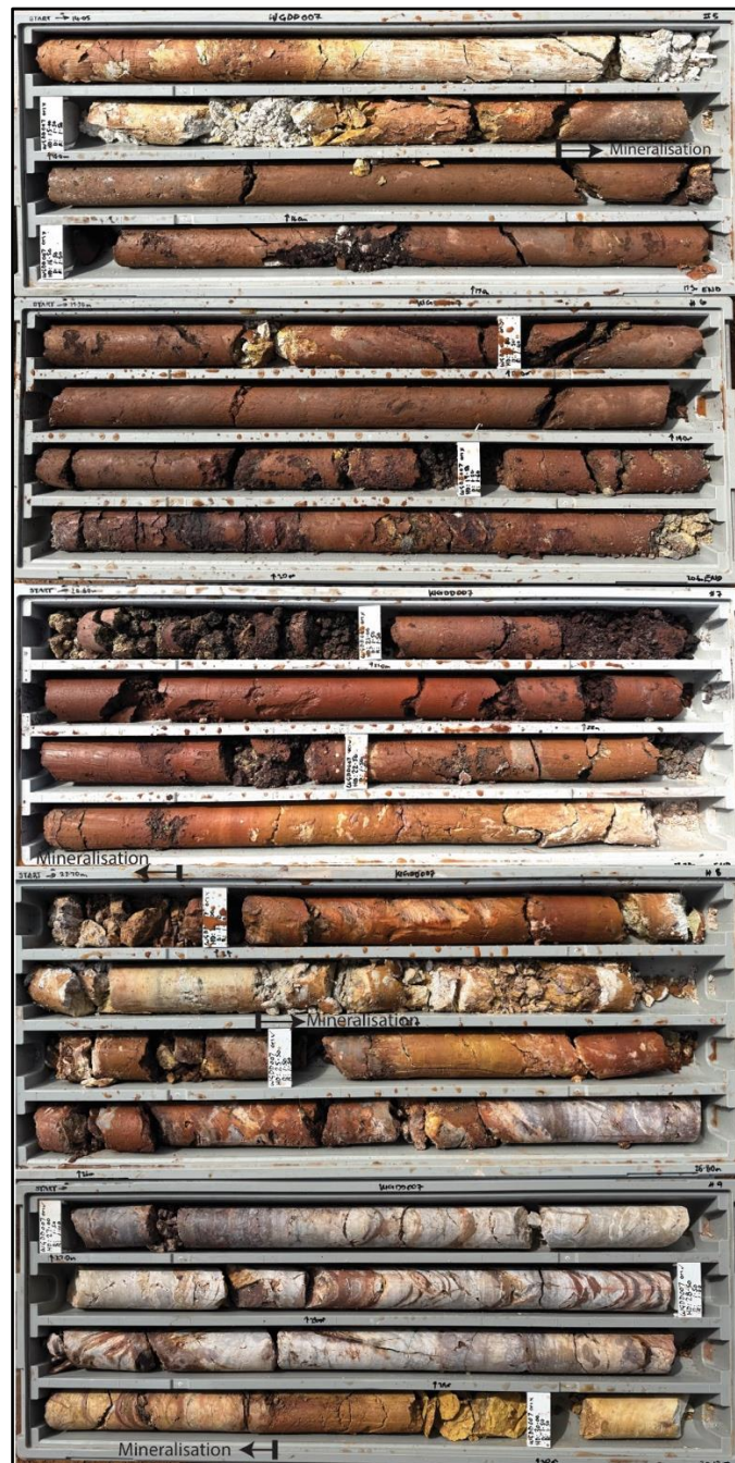
Figure 2. WGDD006: interval 14.05-30.12m: Hematite-goethite altered BIF and brecciated chert mineralisation from the Eagle deposit.
