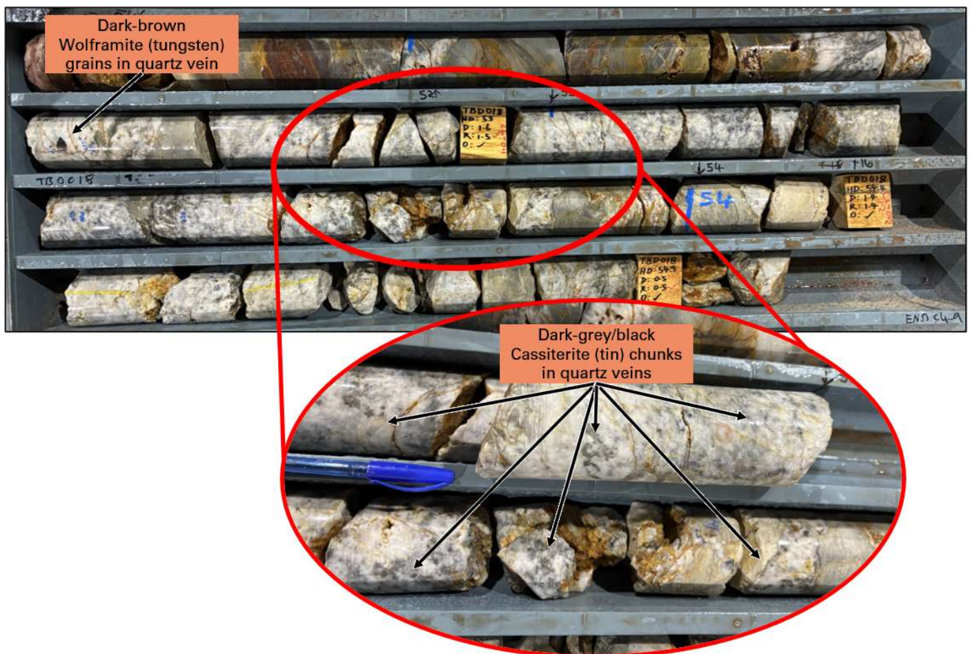
Figure 2: Top: Photo of HQ drill core in core trays from diamond drill-hole TBD018 with wide quartz-cassiterite (tin) veining shown between ~51.6m-54.9m and wolframite (tungsten) grains. Bottom insert: Magnification of the strongly mineralised vein at ~53m and 53.8m where abundant, large cassiterite (tin) chunks are visible in the core as dark grey/brown/black zones in quartz and iron-oxide veins. NB: Cassiterite is 78.7% tin – assays are pending.
