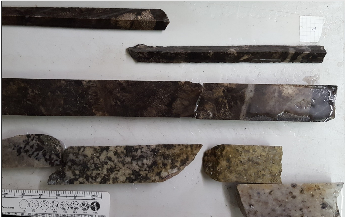
Figure 5: Photos of core from Sadisdorf showing the significant textural difference between the Outer (top) and Inner (bottom) greisens (source CSA, 2017).
