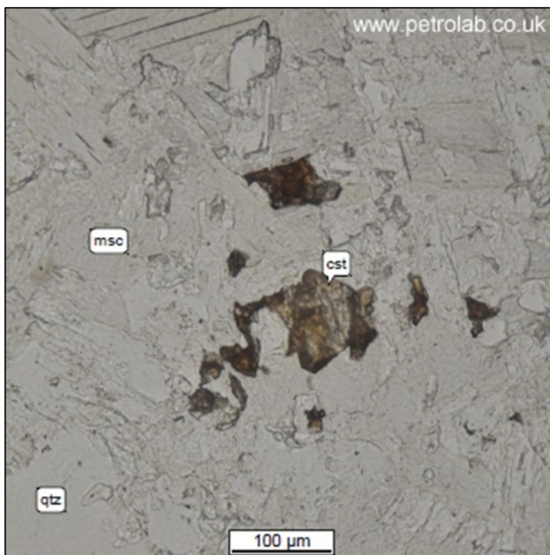
Figure 10: Photomicrograph of coarse-grained quartz and muscovite with fine-grained interstitial cassiterite. Sample C17-15
