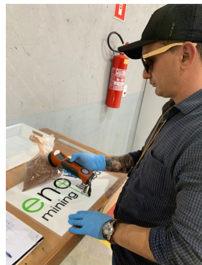
Figure 4: Magnetic susceptibility test for highly magnetised kamafugite samples
