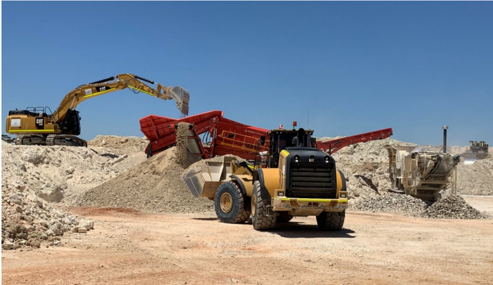
Figure 4 – Screening and Crushing on the Jaurdi ROM pad.
