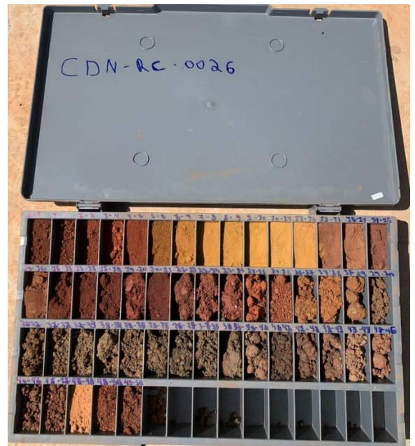
Figure 11: Variegated colour of drill cuttings implying changes in lithology across undifferentiated sediment, laterite, kamafugite
