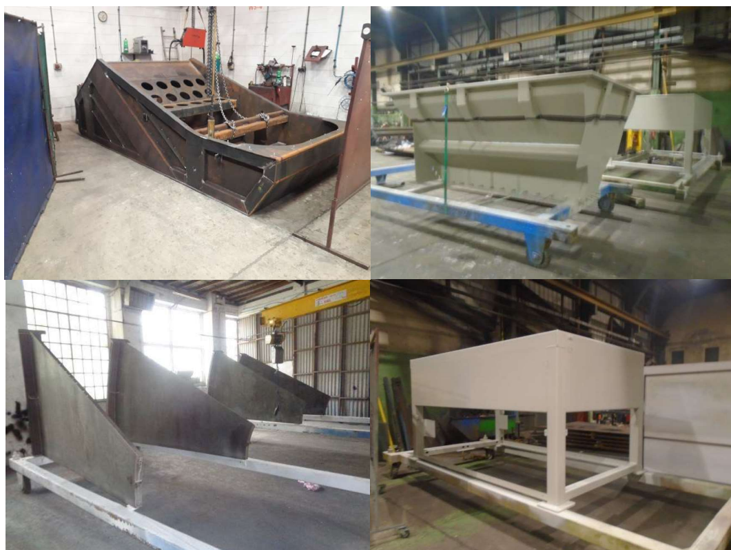
CAPTION: Fabricated sections of the Ardmore modular process plant at CDE Global.
