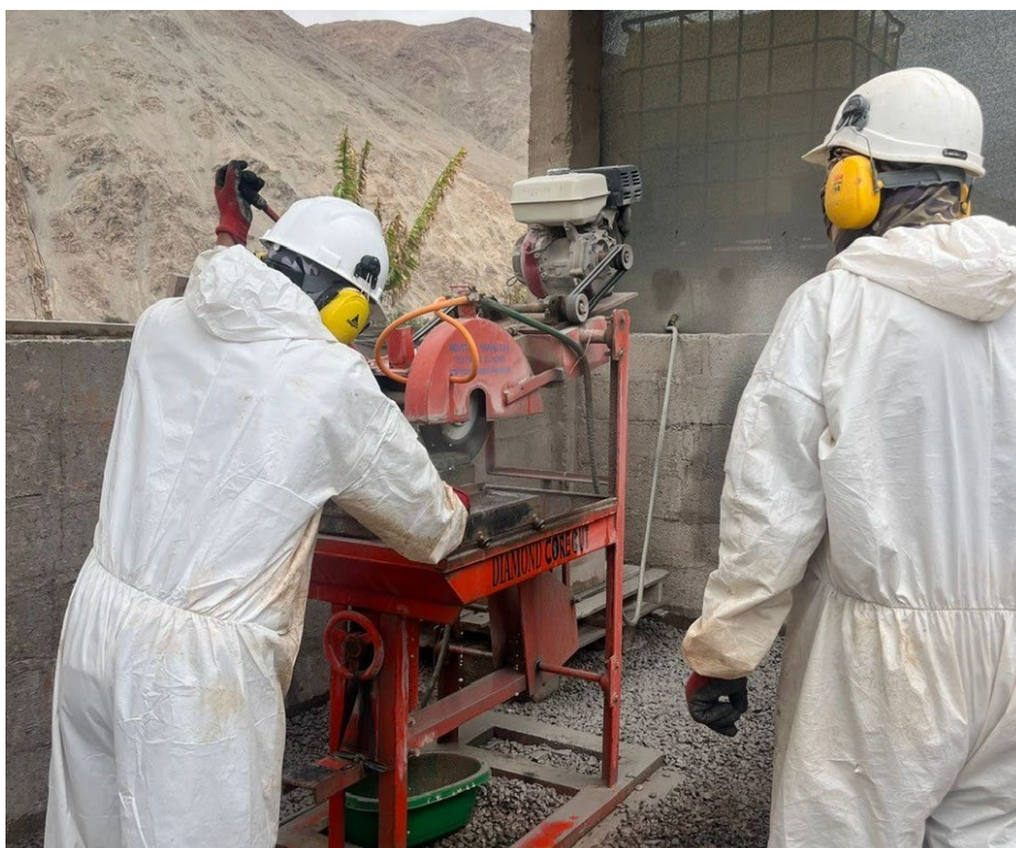
Figure 2: Cutting and logging of drill core has commenced with samples to be processed by ALS in Lima, Peru. Assays are due for release in July / August 2025.
