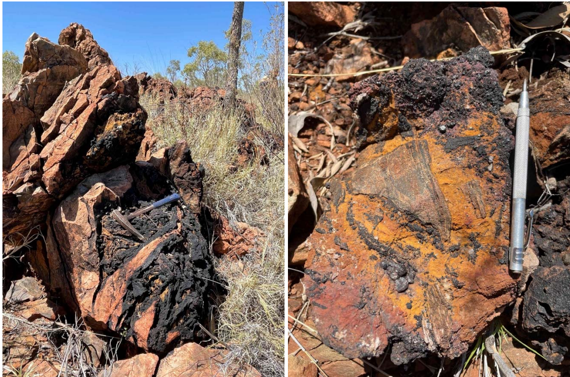
Plate 2: Brecciated metasandstone with black silica-haematite and manganese oxides and goethite on GW Structure, rock chips from this location returned 3.86ppm and 1.61ppm gold.
