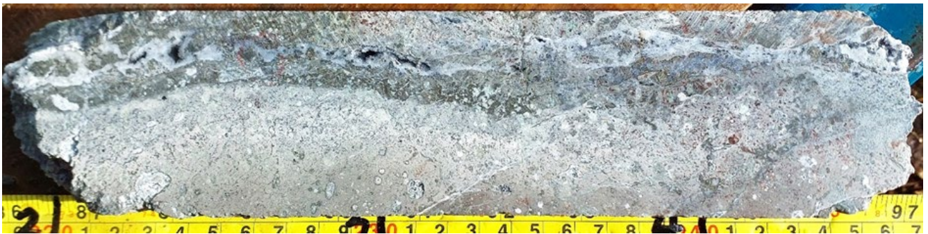
25VDD002_199.58-199.83m. From Sample No. 386656, 199.32-199.9m (0.58m), 26.4 g/t Au, 39.70 g/t Ag. Colloform banded and crustiform chalcedonic silica veins. Open spaces with drizzly quartz. Blebby and fine pyrite, sphalerite and galena-tennantite-tetrahedrite. The host lithology is a vesicular basalt and silica-clay-altered. Disseminated and bebbpy pyrite halo to the veins.
