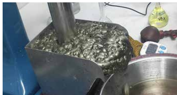
Photo 7: Photograph showing a batch flotation test of the PCZM supergene ore at Maelgwyn.
