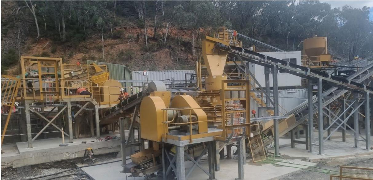
Figure 6 Reward gravity gold plant looking over the 2 jaw crushers and the impact crusher
