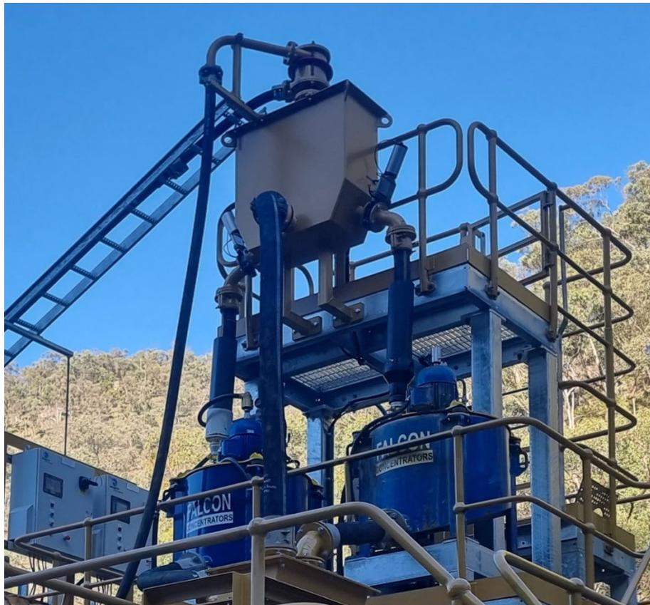
Figure 3 Reward gravity gold Falcon concentrators
