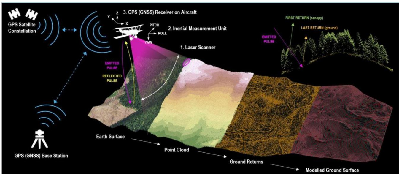
Figure 4: A schematic representation of how LiDAR works (copied, and unmodified, from the GeoCloud website).
