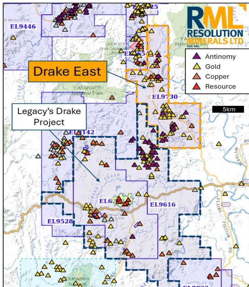
Figure 2: Location map sourced and modified from the NSW Government interactive MinView web map application. The Drake East Project area is shown with a orange dashed line. The Legacy Drake Project area is shown with a dashed dark blue line. The Drake/Drake East projects area hosts over a hundred antimony, gold, silver, and copper occurrences. Many of these are classified by the NSW Geological Survey as non-JORC Code resources.
