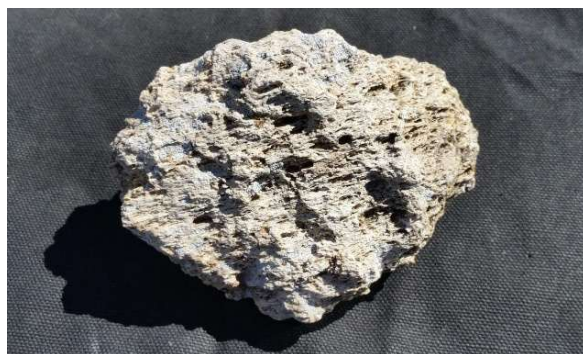
Pozzolans – naturally occurring volcanic materials used in ancient Greek and Roman construction
