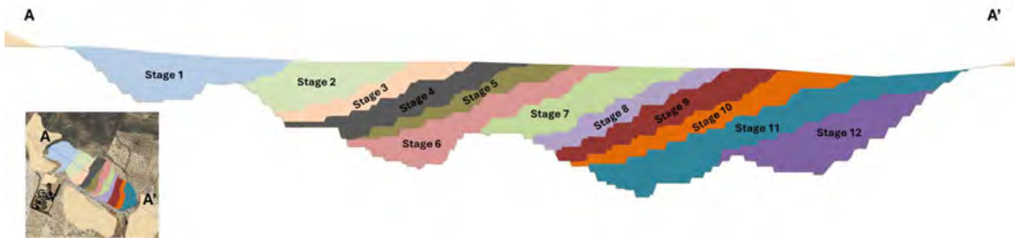
Figure 7-4 – DFS Pit Long Section Showing Mining Stages
