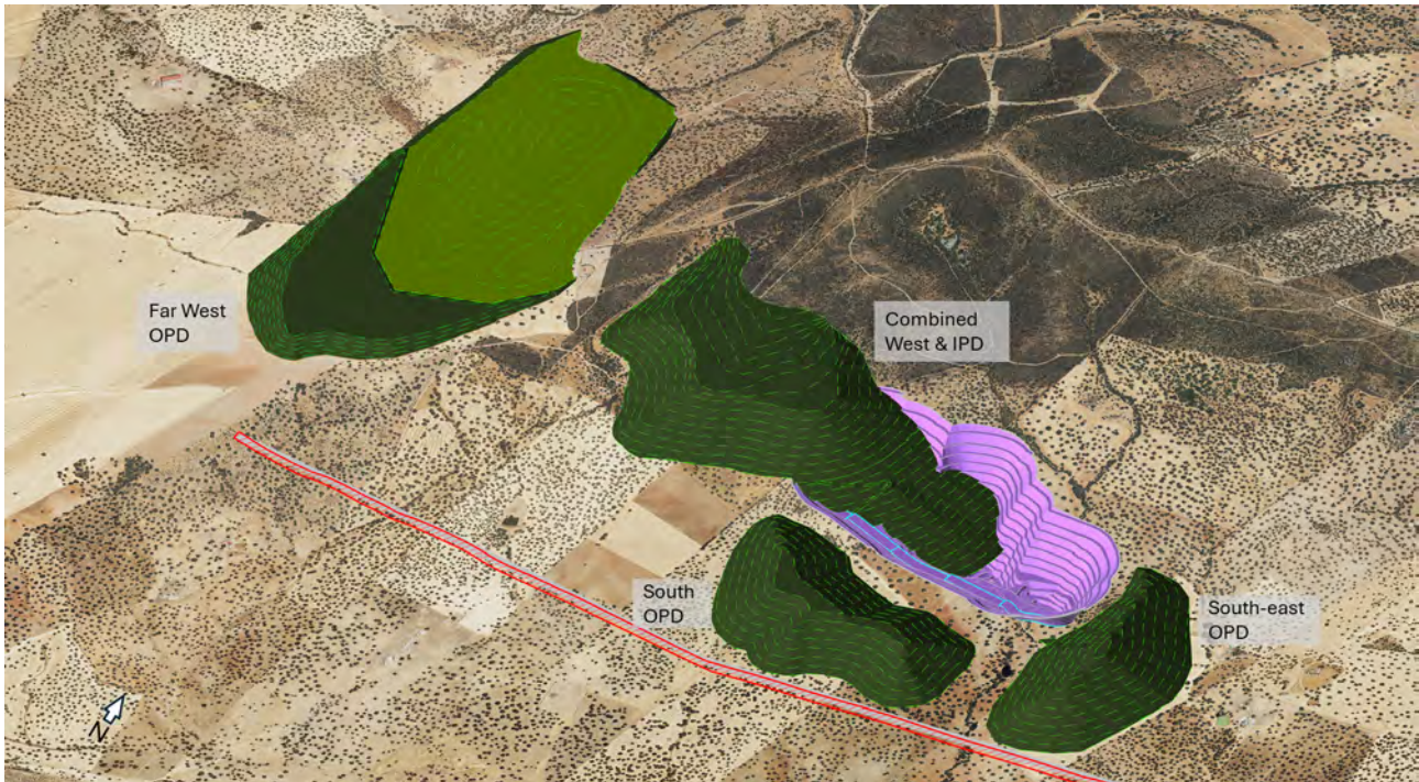
Figure 5-31: Final Landform of Rehabilitated WRF and TSF
