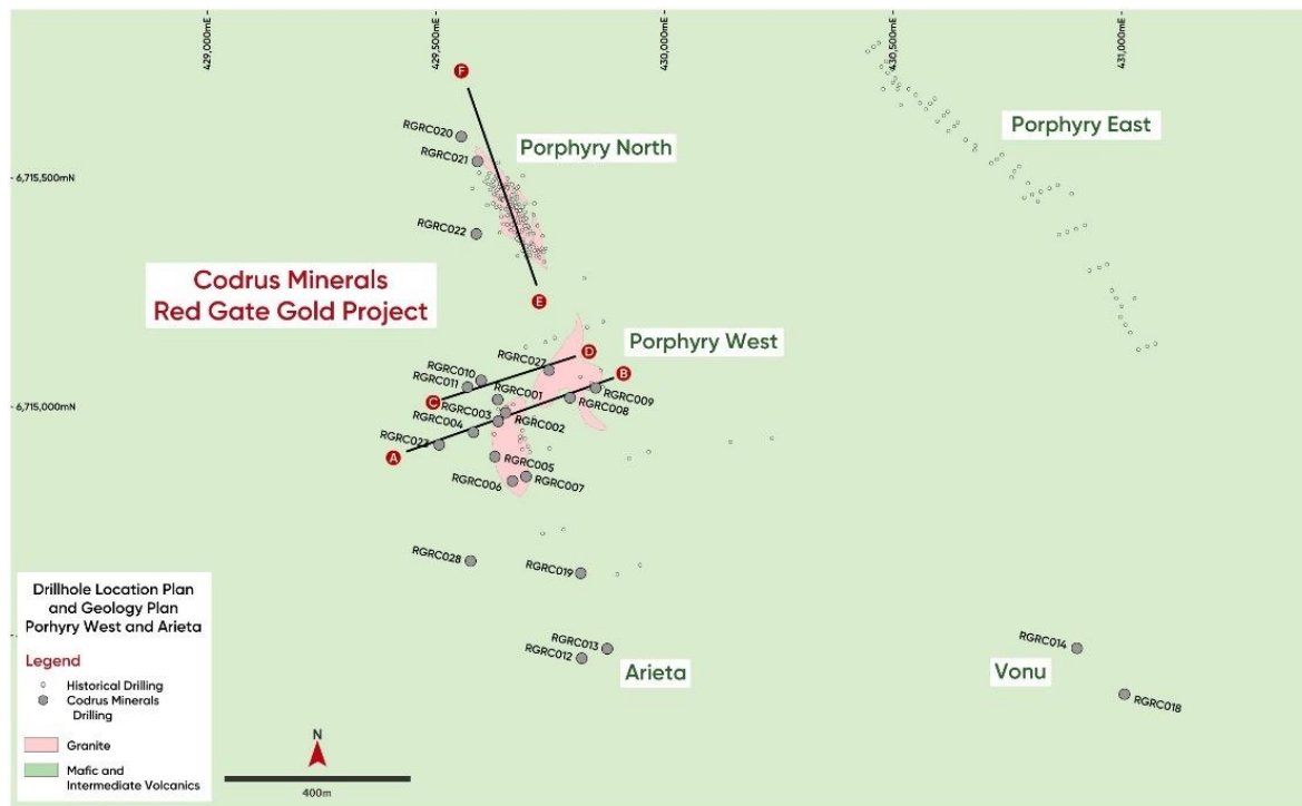
Figure 4. Plan of drill collars at Red Gate Prospects (excluding Grunters)
