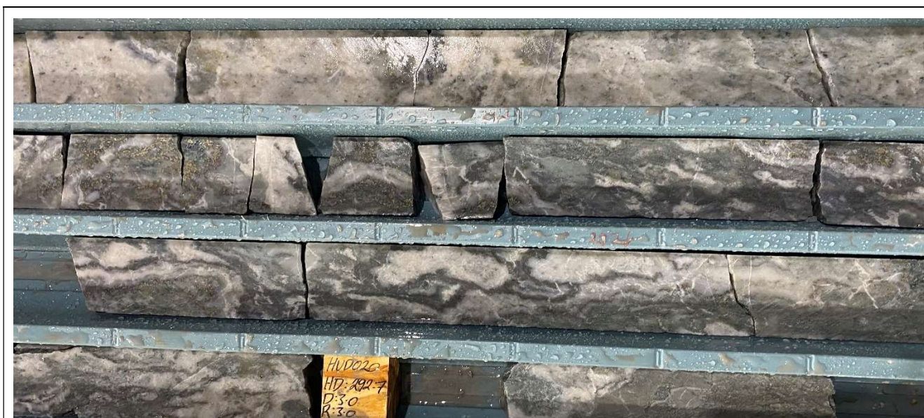
Photo 2 – Cullarin Gold Project - Hume Target – Drillhole HUD020 – 290-293.5m – intense, banded quartz-carbonate-veining with sphalerite & galena.
