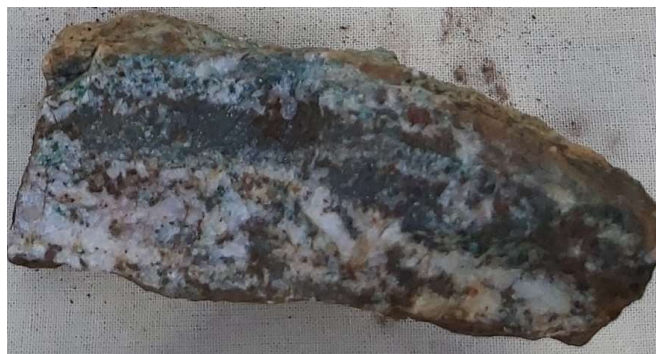
Photo 4 - EL6064 - Christmas Gift - 11.0% Cu, 0.11g/t Au, 24g/t Ag. Quartz, stained with malachite, peppered with malachite on freshly broken surface and also contains fresh disseminated sulphide - pyrite & chalcopyrite. Narrow (~1cm) band suspected chalcocite. Width of view 15cm.
