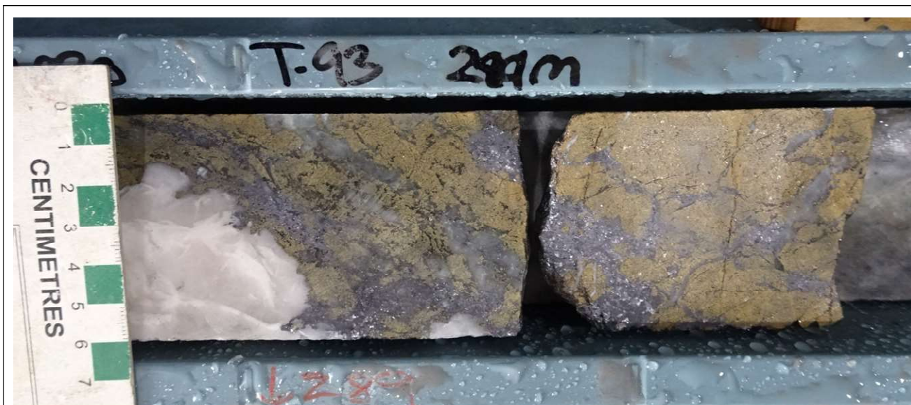
Photo 1 – Cullarin Gold Project - Hume Target – Drillhole HUD020 – 287.5m – massive sphalerite & galena.
