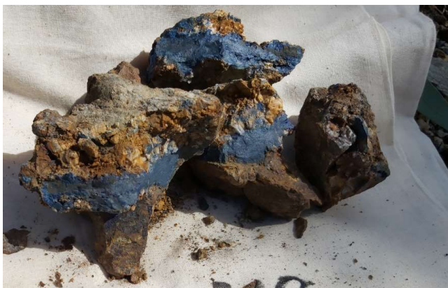
Photo 3 - EL6064 - Monarch - 26.1% Cu, 0.41g/t Au, 29g/t Ag. Spectacular assay result from the >1cm azurite vein and may also contain some chalcocite. Width of view 20cm.
