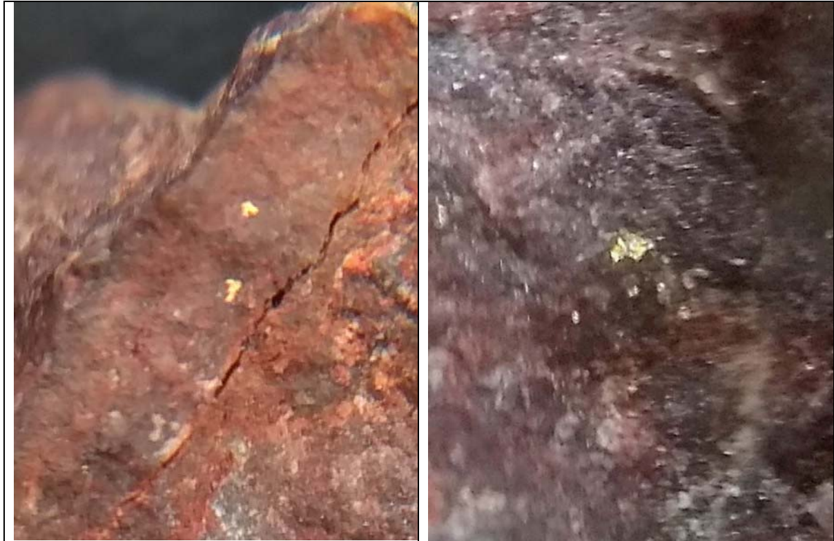
Photo 2 Visible Gold in Sulphide Breccia; Morena Prospect
