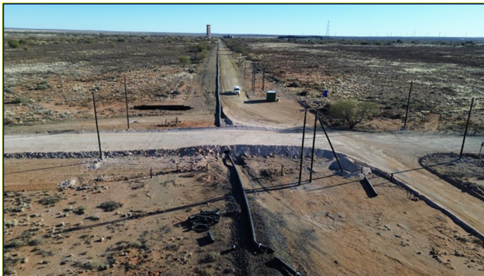
Photo 1: Dewatering Pipe and Overhead 11kV to TSF.
