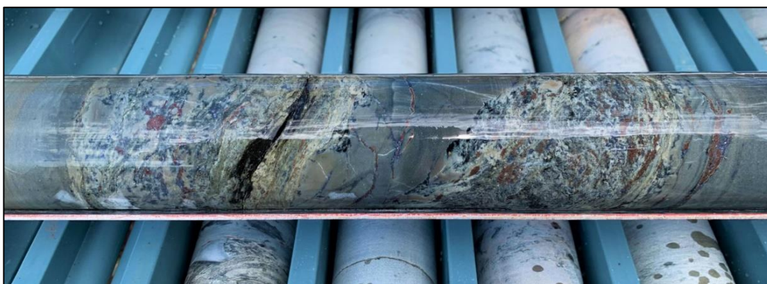
Figure 1: 40cm long drill core (124m downhole) showing bands and veins of blue-grey galena (lead) and maroon-brown sphalerite (zinc) mineralisation.
