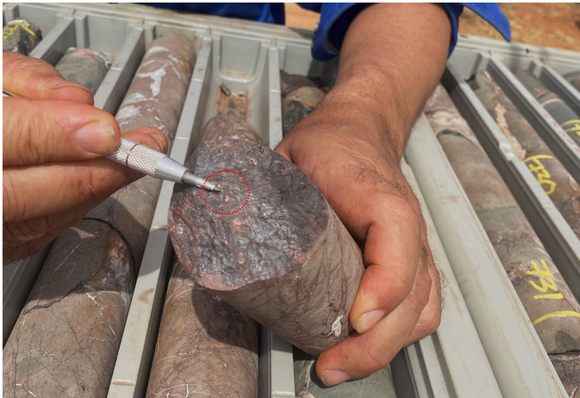
Figure 6: Slickensided parting KNRDD002 with fine native copper indicated at approximately 732.5m down-hole.
