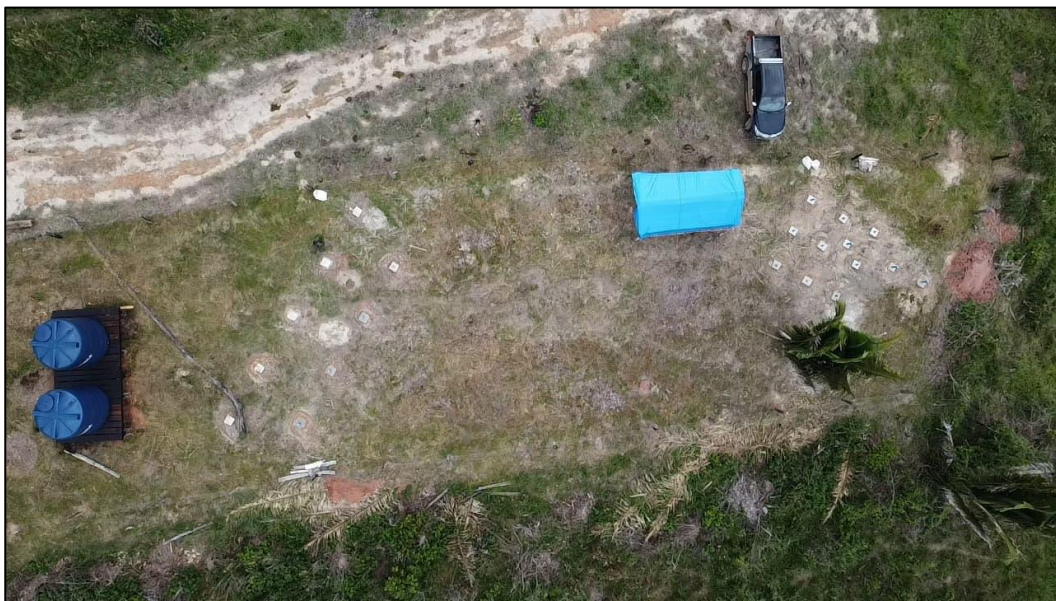
Figure 12. Ema permeability field trial setup. White squares are the concreted collars of the drill holes which will be injected with water and/or lixiviant pumped from the blue storage tanks. Two separate test zones have been developed, one with shallow holes drilled to 5.7m depth (adjacent to car) and test zone 2 with both injection and extraction holes drilled to 10m depth adjacent to the 2 10,000 litre water storage tanks.
