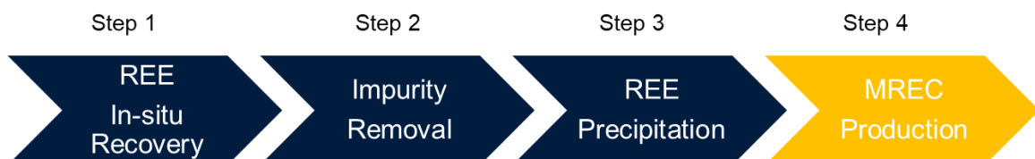
Figure 6. Simple 4 step process flow sheet for ionic clay MREC production at Ema Project
