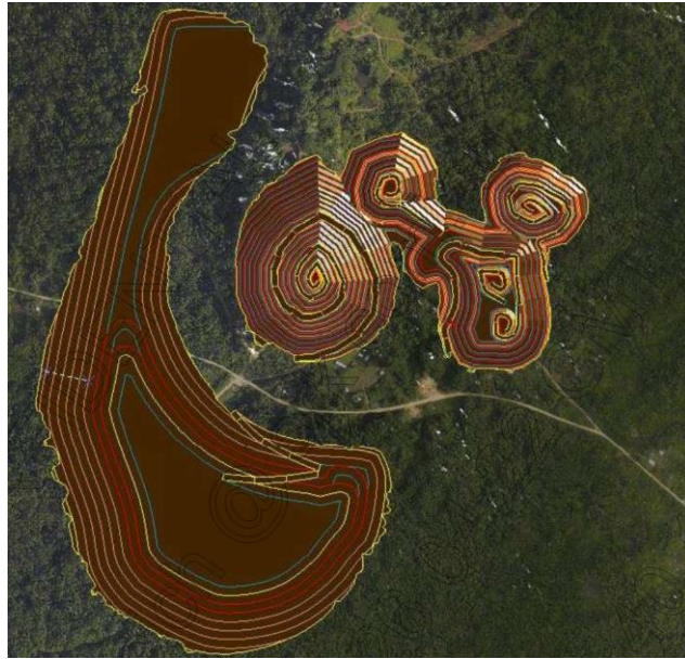
Figure 15 Kulumadau Final Pit Design
