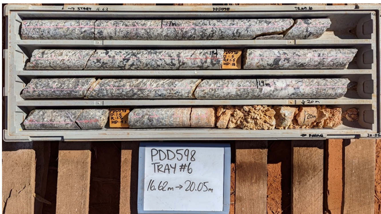
Figure 1 – Example of drill core taken from the upper zone of the Cade Deposit illustrating the relatively homogenous mineralised pegmatite and some weathering on fractured sections (Hole ID PDD598).
