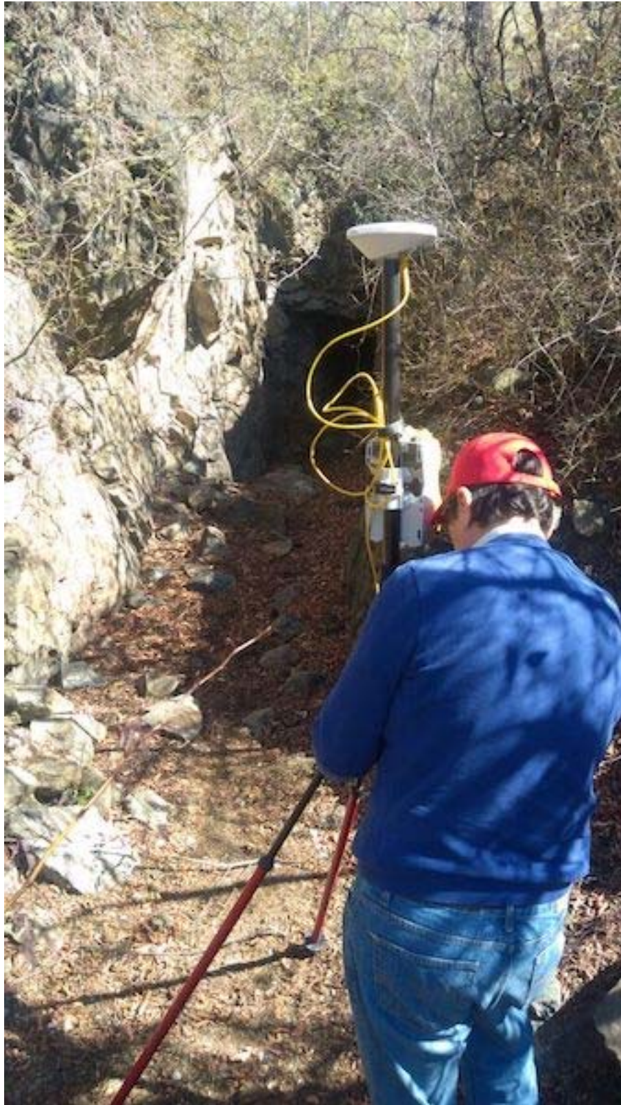
Photo 3: Surveyors utilising GPS technology to establish permanent survey stations to support topographic mapping over the Las Tapias Mine property.
