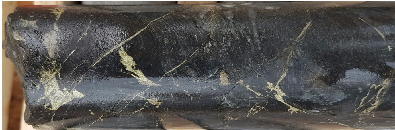
Plate 1 Copper mineralisation hole 16WD02. (Core length approx. 20cm)
