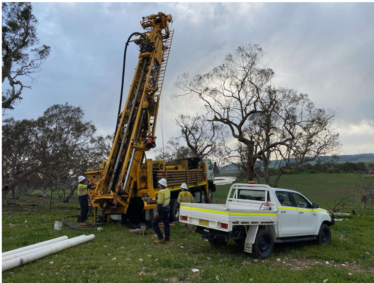
Hume North RC Percussion Drilling HUR001
