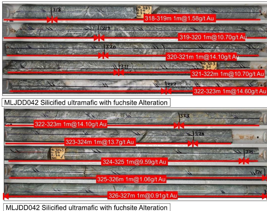
Figure 11. Drillhole MLJDD042 from 318m to 327m showing silicified ultramafic with fuchsite alteration
