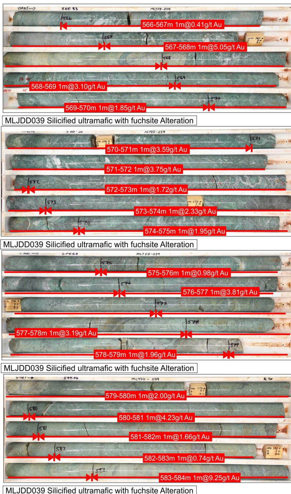
Figure 13. Drillhole MLJDD039 from 566m to 584m showing silicified ultramafic with fuchsite alteration
