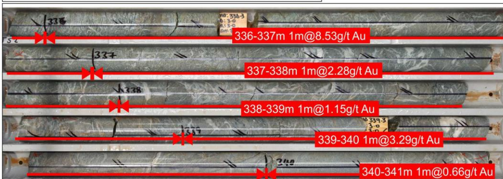
MLJDD042 Silicified ultramafic with fuchsite Alteration
