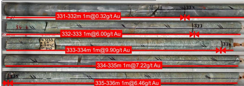
MLJDD042 Silicified ultramafic with fuchsite Alteration
