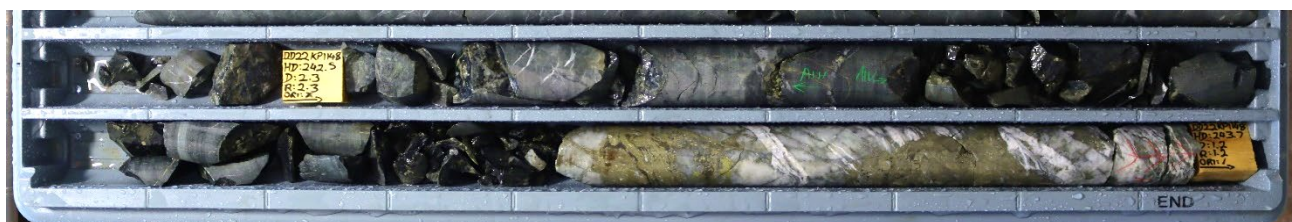
Figure 4: DD22KP1094 highlighting quartz-sulphide veining between 162.6m – 164.65m with associated dark green chlorite alteration. Total sulphide abundances estimated at 60% comprised of 20% chalcopyrite and 40% pyrite.
