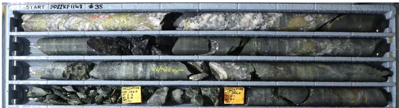
Figure 5: DD22KP1148 with quartz-sulphide vein between 243.2m - 244.8m comprised of 30% pyrite and 10% chalcopyrite. Sulphide stringer veins and chlorite alteration are observed in the footwall to the vein.
