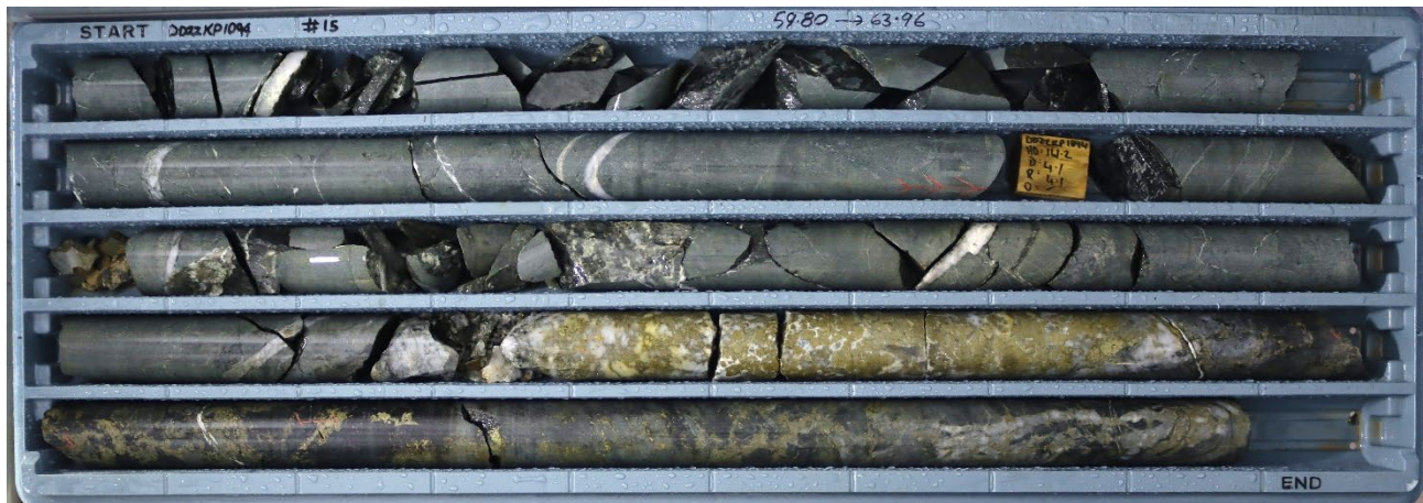
Figure 4: DD22KP1094 highlighting quartz-sulphide veining between 162.6m – 164.65m with associated dark green chlorite alteration. Total sulphide abundances estimated at 60% comprised of 20% chalcopyrite and 40% pyrite.
